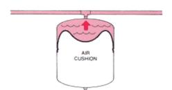
When hot water is used in the system....the pressurized air cushion forces hot water back into the system for use....not waste.
